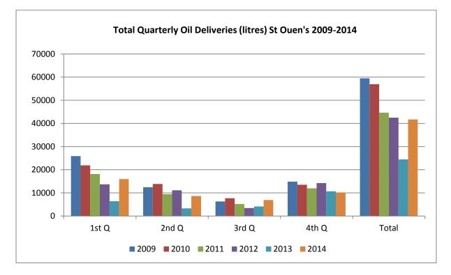
The cavity wall and loft insulation was completed in the  $3^{rd}$  Quarter of 2010 and the boiler upgrades in the  $4^{th}$  Quarter of 2011.
