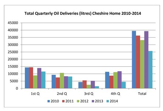
The cavity wall and loft insulation was completed in the 1<sup>st</sup> Quarter of 2011 and the main boiler upgrade in the 2<sup>nd</sup> Quarter of 2012. The hydrotherapy boiler was not upgraded until September 2015.
