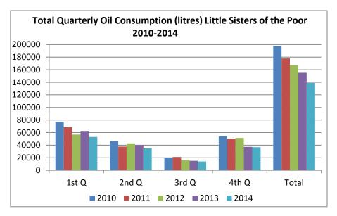
The cavity wall and loft insulation was completed in the 1<sup>st</sup> Quarter of 2011 and the boiler upgrades in the 3<sup>rd</sup> Quarter of 2012.
