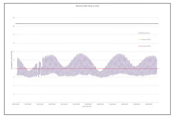
Figure 14: Borehole BH2/16 Vibrating Wire Piezometer Data (23m bgl) – Groundwater Level
