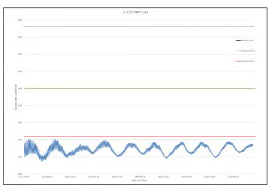
Figure 7: Borehole BH2/09 Vibrating Wire Piezometer Data– Groundwater Level
