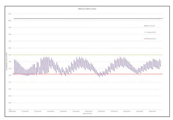
Figure 9: Borehole BH2/15 Vibrating Wire Piezometer Data (20m bgl) – Groundwater Level
