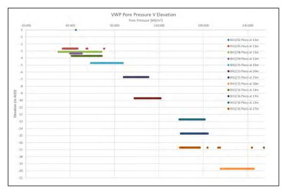
Figure 16: Vibrating Wire Piezometer Results - Pore Pressure v Elevation
