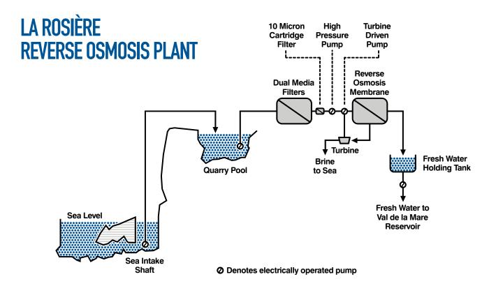
A deep sea water intake shaft and tunnel constructed below the mean low tide level on the foreshore allows sea water to be pumped at all states of the tide, which can vary by as much as 12m. A macerator device in the sea water intake shaft chops up seaweed and other large matter. The sea water is discharged and stored into the quarry pool, which allows settlement of any unwanted debris rather than it floating to the surface.
