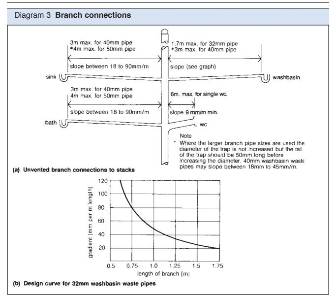
**1.10** Branch pipes from more than one ground floor appliance may discharge into a stub stack. (See paragraph 1.26.)
