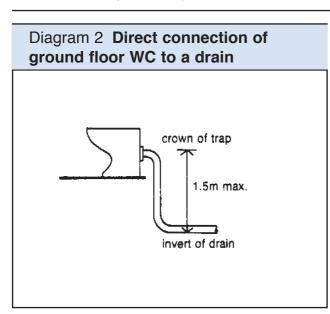
**1.6** If the appliances are on the ground floor the pipe(s) may discharge to a stub stack or discharge stack, directly to a drain, or (if the pipe carries only waste water) to a gully. (*See paragraphs 1.9 and 1.2*).
