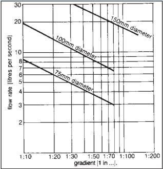
**2.11** A drain carrying only waste water should have a diameter of at least 75mm and a drain carrying soil water or waste water containing trade effluent a diameter of at least 100mm.
