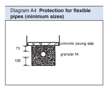
**A15** Where flexible pipes are not under a road and have less than 0.6m cover they should, where necessary have concrete paving slabs laid as bridging above the pipes with at least 75mm of granular material between the top of the pipe and the underside of the slabs (see *Diagram A4 and paragraphs 2.9 and 2.18*).
