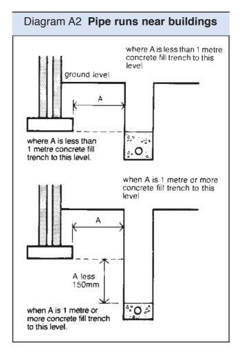
(b) where the trench is further than 1m from the building, the trench is filled with concrete to a level below the lowest level for the building equal to the distance from the building, less 150mm.
