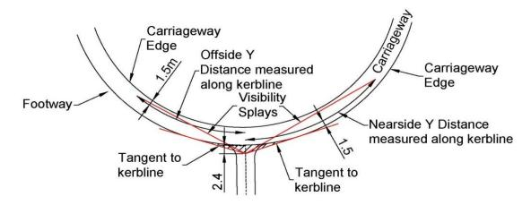
Figure 13 – Measurement of Access on the Outside of a Curving Highway
