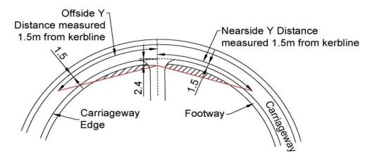
Figure 14 – Measurement of an Access on the Inside of a Curving Highway
