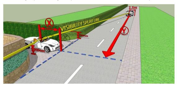
Figure 9 – Measuring Visibility Splay Area to the Offside
