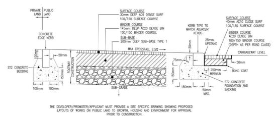
Figure 6 – Medium Duty Footway Construction
