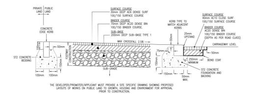
Figure 2 – Light Duty Footway Specification
