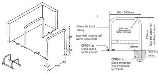
Figure 17 – Cycle Parking Stand Specification
