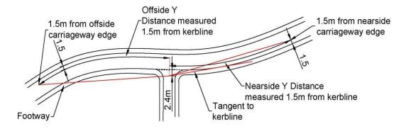
Figure 15- Measurement of Access on the Inside and Outside of a Curving Highway
