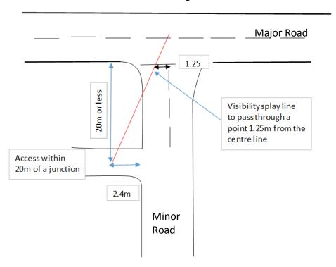
Figure 12 – Visibility from an Access within 20m of a Junction
