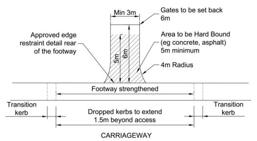
Figure 5 - Continuous Footway across an Access
