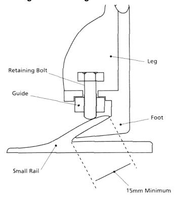
Diagram 9 - Typical parallel Claw fitting
