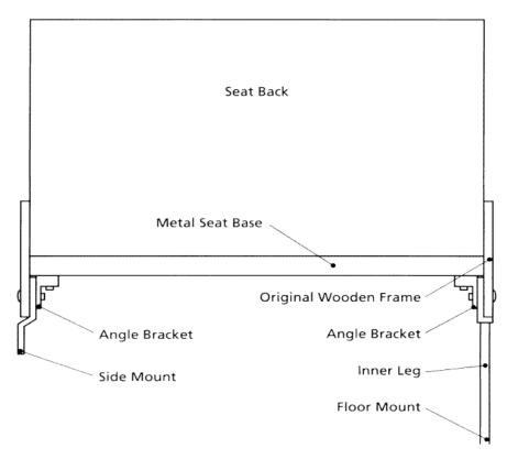
Diagram 4 - Wooden framed seats with a metal base (enlargement of reinforcement)
