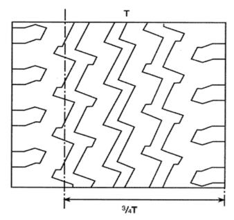
In this case the lateral grooves are the same depth as the circumferential groove and are included in the 3/4 measurement
