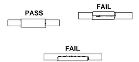
Guidance on sleeved repairs of metal brake pipes (sleeving is not acceptable on plastic brake pipes)
