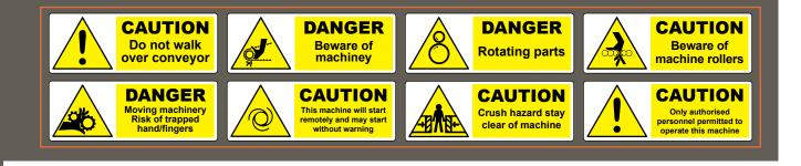
All machinery should be marked with highly visible and indelible labels to provide warnings and raise awareness relating to the safe use of equipment. Pictograms are often used to represent particular hazards via symbols and pictures.
