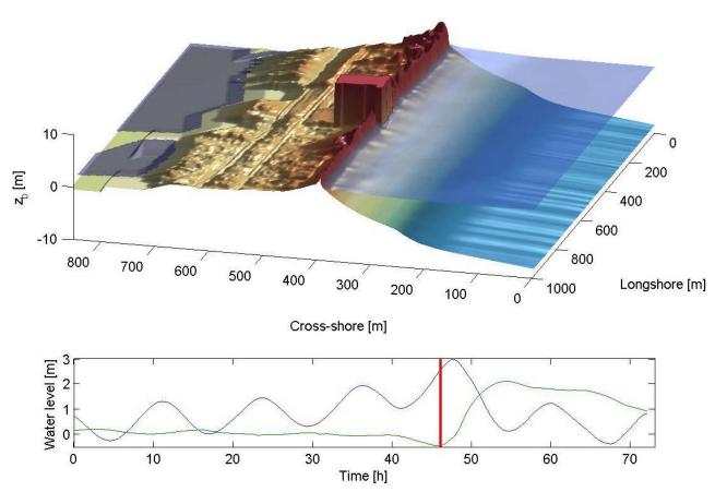
Figure 16: Example of a 2DH XBeach simulation.
