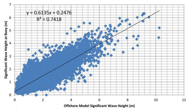
*Figure 12: Significant wave height from offshore model against significant wave height at wave buoy.*
