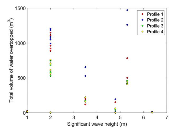
*Figure 30: Mean total overtopping volume for each profile for a selection of scenarios simulated.*
