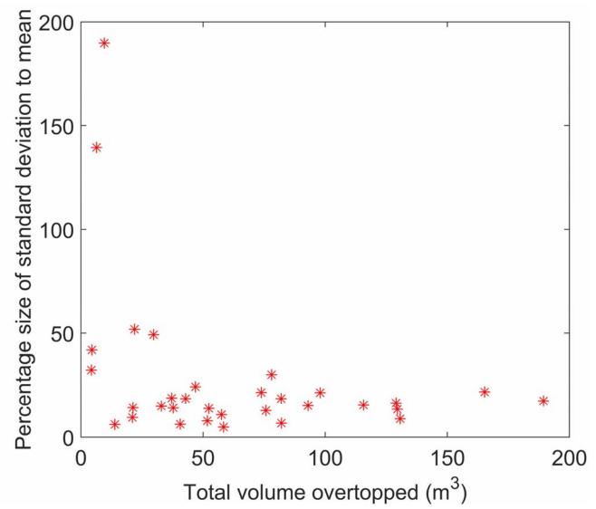
*Figure 32: Mean total volume for a selected scenario against the percentage size of the standard deviation against the mean total volume.*
