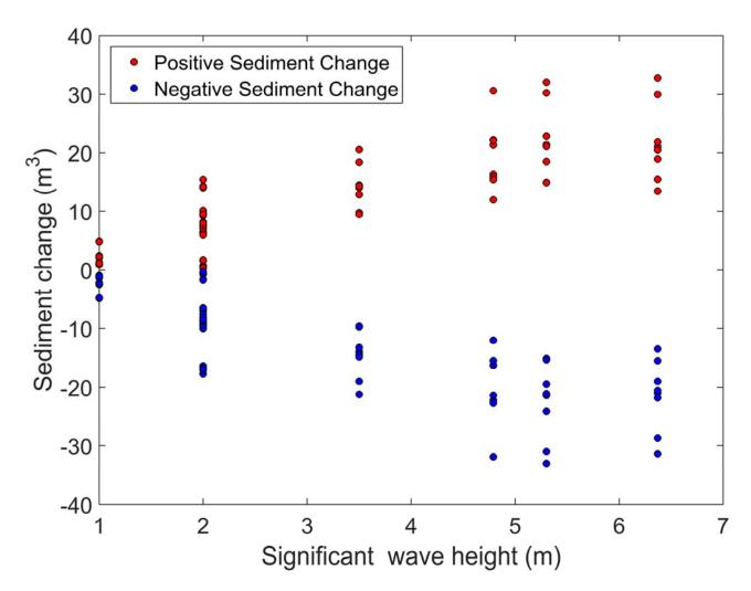
*Figure 26: Positive (red dots) and negative (blue dots) sediment change across the whole profiles against significant wave height used in the extreme events.*
