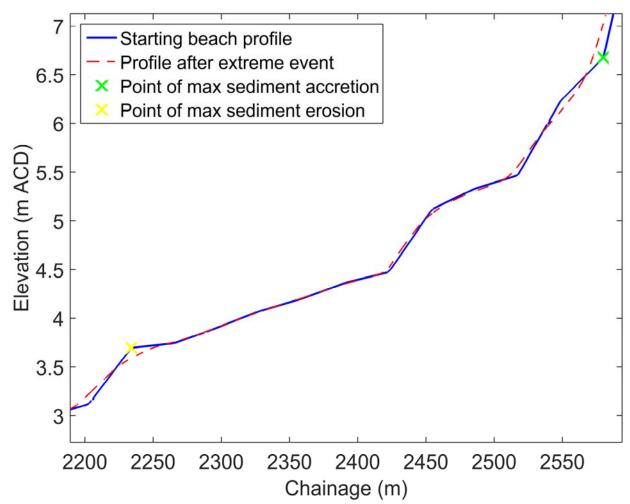
*Figure 29: Close up of profile 2 showing locations of max and min sediment change, both the starting profile (blue) and the end profile (dashed red) are shown.*
