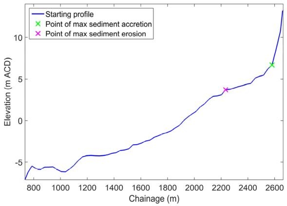
*Figure 28: Profile two showing locations of max and min sediment change for greatest sediment change (Scenario 10).*
