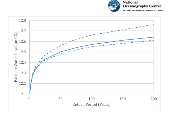
Figure 9: Linear plot of return period against extreme water level up to a 1 in 200-year event, the solid line represents the return period values and the dashed lines indicate the 95% confidence intervals.
