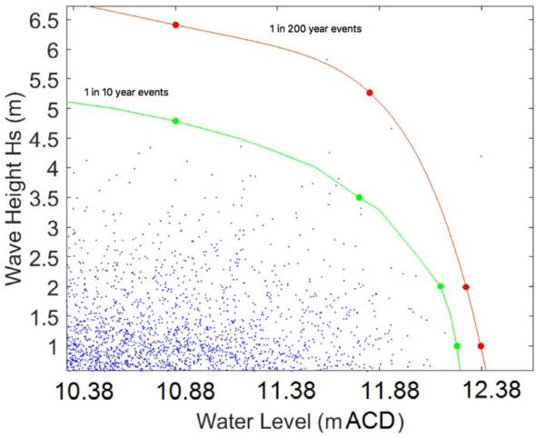
*Figure 15: Close up of joint probability curves showing the 8 combinations selected for simulation. The green line shows 1 in 10 year values and the red represents 1 in 200 year events.*
