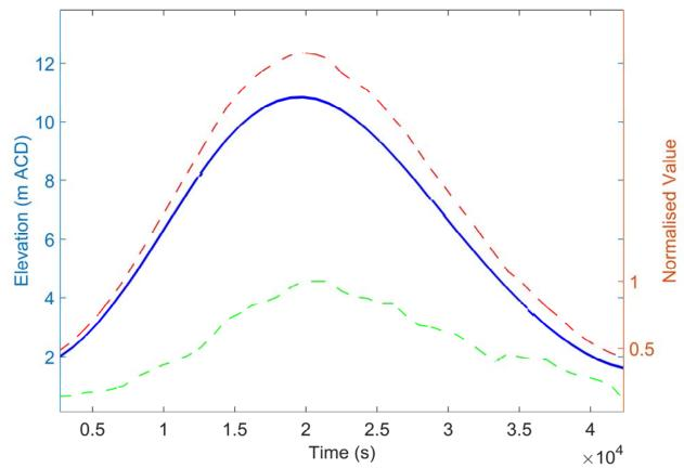
Figure 24: Diagram showing example of producing storm tide, solid blue line is a predicted MHWS curve for Jersey, green dotted line is the representative surge curve, and red dashed line is the output storm tide for inclusion in XBeach simulations.
