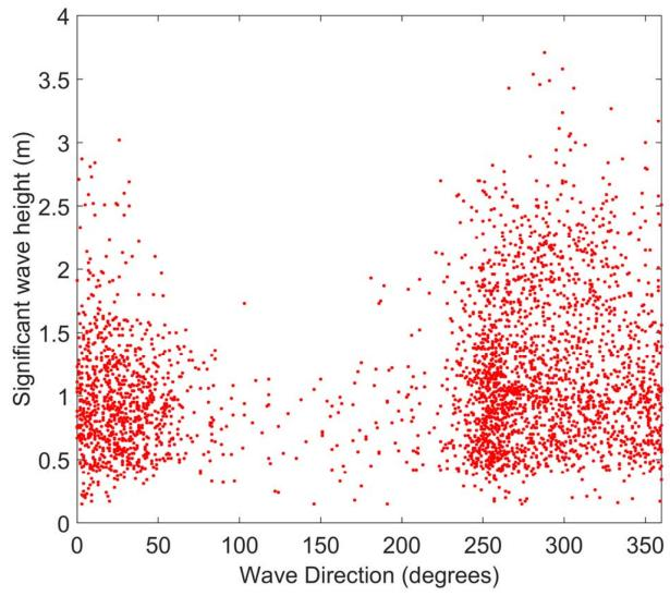
Figure 23: Wave direction against significant wave height at wave buoy
