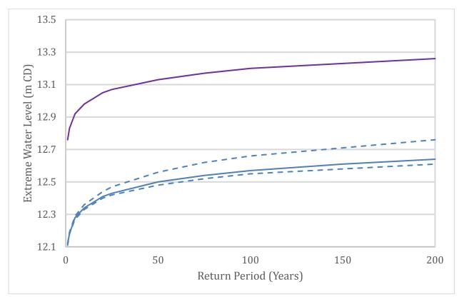
Figure 10: Impact of 0.65 m of SLR on return period values for Jersey. Purple shows the extreme water level for a given return period for an increase in mean sea level of 0.65 m. The blue line shows the present-day relationship with associated confidence interval
