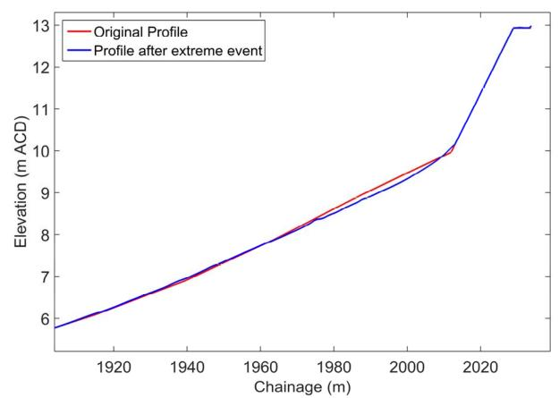
*Figure 25: Example of changes to beach morphology due to an extreme event of a 1 in 200 RP with an WL of 6.45 m, Hs of 2 m and a Dir of 270 with a Tp of 19.7 s.*
