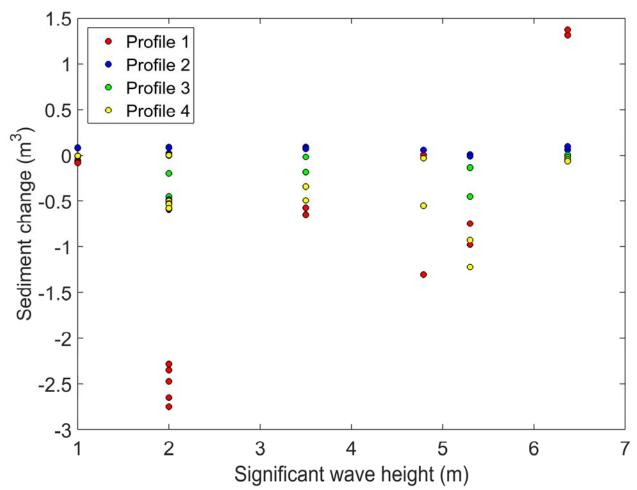
*Figure 27: Total sediment change for every scenario showing sediment lost or gained from beach profile.*
