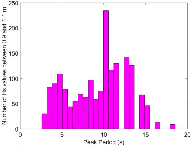
*Figure 22: Histogram for all Hs values between 0.9 m and 1.1 m for the wave buoy between 2011 and 2012.*
