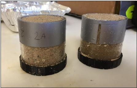
Figure 2. 0-5cm and 5-10cm cut sample cores prior to cleaning and desiccation.
